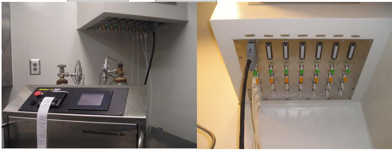
Distribution Plate (Part #: CSI-ROOM015) Unit Dimensions for 14 chambers: 16.0" x 56.0" Unit Weight: 15 lbs
