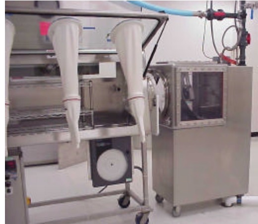
Cloridox-Docking Station Dimensions 45"W x 64"H x 24"D (8 cubic ft. chamber) Weight 300 lbs
