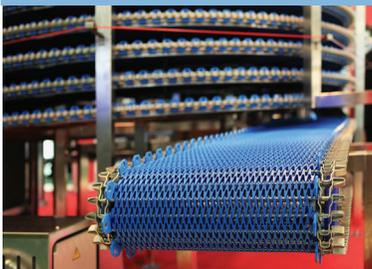
A 25,000 ft<sup>3</sup> Spiral Freezer used at a frozen sausage production facility had a consistent listeria problem, producing positive environmental swabs time and again. After one treatment with chlorine dioxide gas, the facility reached 16 weeks without a single positive swab for listeria after swabbing 2-3 times per day. Upon achieving these results, the facility purchased a generator and instituted the use of chlorine dioxide gas on a quarterly basis for preventive decontamination.
