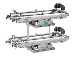
The Flash Flood is a UV-C water treatment device that operates inline with your water system. Ultraviolet light is a superior method of water disinfection because harmful organisms are destroyed simply by light and without the need for any chemicals. Chemical water treatments may result in taste and odor problems, undesirable chemical reactions with substances present in the water, or dangerous handling issues.
