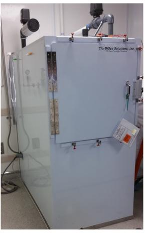
The equipment is available in a variety of sizes to meet your processing needs and can be manufactured with either a single door or double door pass-through orientation. A door interlock system is also available.
