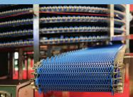
A 25,000 ft3 Spiral Freezer used at a frozen sausage production facility had a consistent listeria problem, producing positive environmental swabs time and again. After one treatment with chlorine dioxide gas, the facility reached 16 weeks without a single positive swab for listeria after swabbing 2-3 times per day. Upon achieving these results, the facility purchased a generator and instituted the use of chlorine dioxide gas on a quarterly basis for preventive decontamination.
