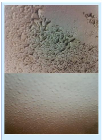
"The two pictures show epoxy coatings that started to blister and peel due to VHP."
