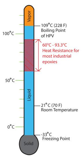
"The cause of hydrogen peroxide's effect on epoxy is partly due to the superheated temperature to which it is vaporized and introduced for decontamination. Most industrial epoxies have a heat resistance limitation between 60°C and 93.3°C (140°F–200°F). Since hydrogen peroxide vapor exits a generator at a temperature of at least 109°C, it can cause damage upon contact with epoxy coatings and surfaces."
